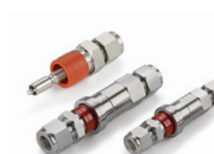
QCLOK® Quick Connectors 1/4", 3/8", 1/2" MAWP: 3,000 psi (413 bar) MAWT: 500°F (260°C)
