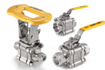
3 Piece Ball Valves - H-500 series MAWP: 3,000 psi (206 bar) MAWT: 450°F (232°C)
