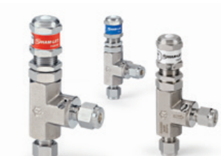
Relief Valves - H-900 & H-900HP series MAWP: 6,000 psi (413 bar) MAWT: 300°F (148°C)
