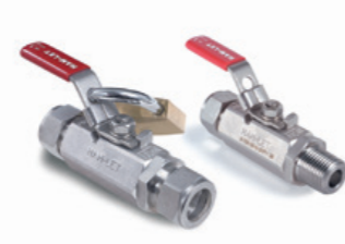
Ball Valves with Locking Device - H-700 series MAWP: 2,000 psi (137 bar) MAWT: 400°F (204°C)
